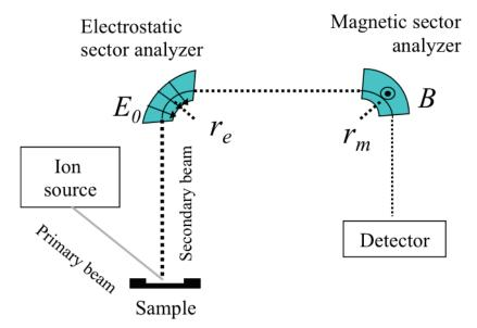
Currently, the more common type of mass spectrometer used in SIMS is the sector field mass spectrometer. This uses an electrostatic sector analyzer coupled with a magnetic sector analyzer. This concept uses the Lorenz force to bend the ion through the electrostatic and magnetic sectors. The Lorenz force is equal to the Centripetal force, which is given by the equation below.
