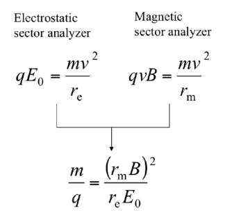
One can use an energy-resolving slit to filter out the unwanted ions from the analysis process, because the unwanted ions will be bent to a different degree. Other types of analyzers include the quadrupole mass analyzer, which separates masses by resonant electric fields, and the time-of-flight mass analyzer, which calculates mass based on the time required to traverse a known distance after a given acceleration.
