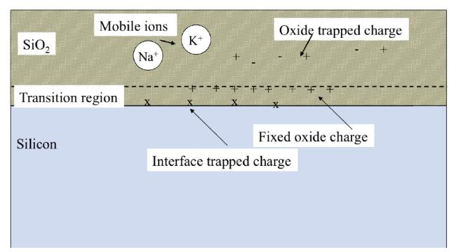
This diagram shows the four different types of charge that can occur in the silicon dioxide and at the silicon/silicon dioxide interface. Mobile ions such as sodium and potassium can be found scattered throughout the silicon dioxide layer. In the presence of an electric field however, they can be attracted to
