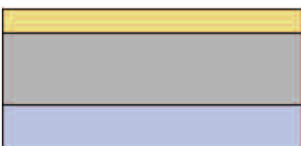
Cover film (OPP 16µm) Resin layer (10-100µm) Support film (PET 38µm)
