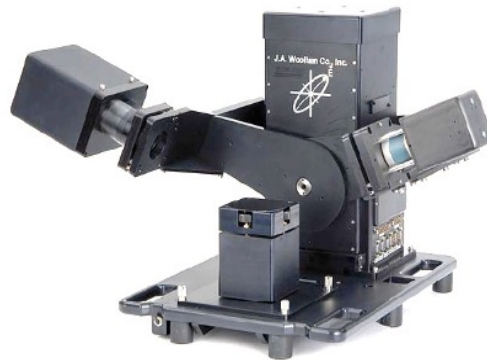
Figure 2- An example of a spectroscopic ellipsometer (courtesy J.A. Woollam Co., Inc.)
