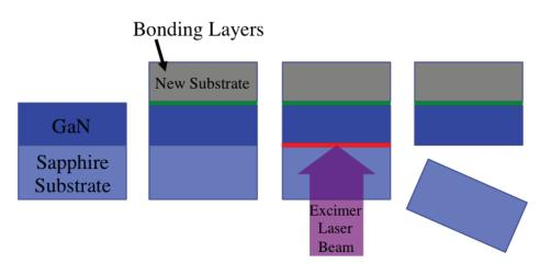
Let's look a little further into how the laser lift-off method works. First, one deposits metal on the receptor and semiconductor wafers. The typical metal is palladium on the receptor wafer, and titanium-palladium-indium on the semiconductor wafer. Second, one bonds the wafers together at low temperatures. This creates a palladium-indium alloy. Third, one focuses laser light through the semiconductor wafer on the
