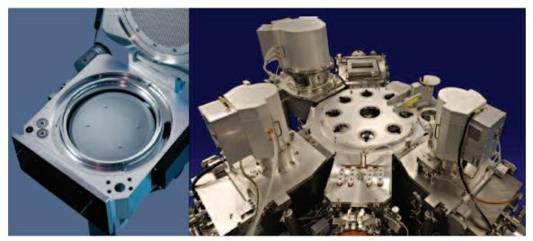
These images show examples of the process chamber and the entire cluster tool for LPCVD. Although these tools are more complex and suffer from slower throughput, the benefits of performing multiple operations together and doing them more uniformly outweigh the disadvantages in most situations.
