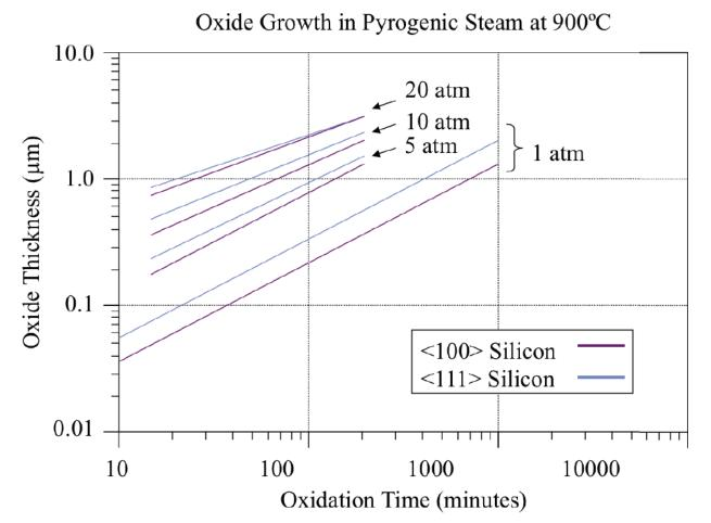
This graph shows the effects of pressure on oxide growth in pyrogenic steam. The graph shows the oxide thickness as a function of oxidation time for several different pressures. Notice that the oxide growth rate increases as the ambient pressure is increased.
