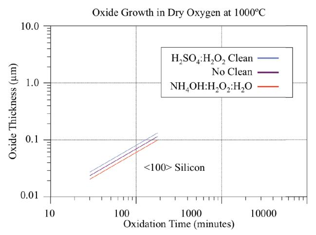
This graph shows the effects of two different pre-treatments, and no pre-treatment of the silicon surface. The sulfuric acid – hydrogen peroxide clean oxidizes the surface, allowing faster oxide growth, while the ammonium hydroxide – hydrogen peroxide – water clean makes the surface more alkaline, reducing the growth rate.
