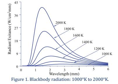
If one plots the radiancy versus wavelength, the relationship can be seen (Figure 1). Notice that as the temperature increases, the peak in the radiancy moves toward shorter wavelengths.
