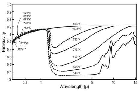
Figure 3. Silicon emissivity.
