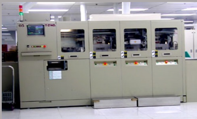
Figure 1- Image of an "Auto Mold" transfer molding system from Towa.
